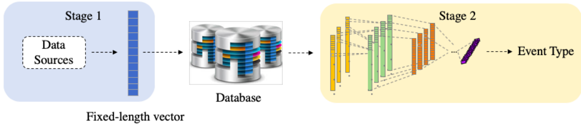
Figure 3. System overview. The input are raw data from smartphone embedded sensors. In practice, smartphone keeps running stage 1 converting massive data into fixed-length vectors and stores them into the database, once the user has the risk of exposure to virus, the stage 2 would fetch vectors from database and estimate the event type.
